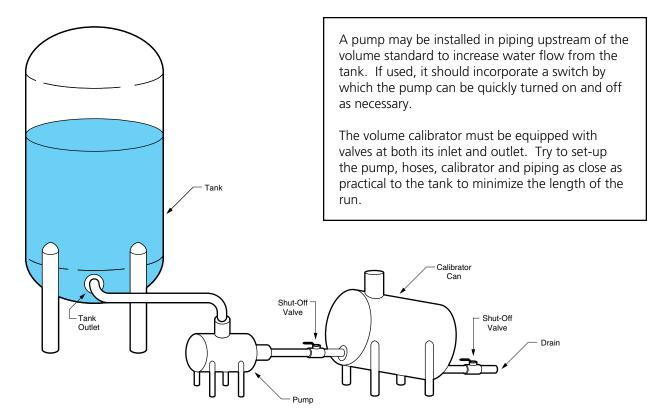
Recommended "Out" Calibration Procedure Using Volume Standard (Calibration)
