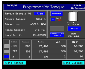
LP3 Drill Down Detail The color touch screen allows quick access to details including engineering units selections, tank capacity and communications status. Configuration settings are readily visible from each tank detail screen. (Access to these settings is password-protected to ensure data integrity.)
